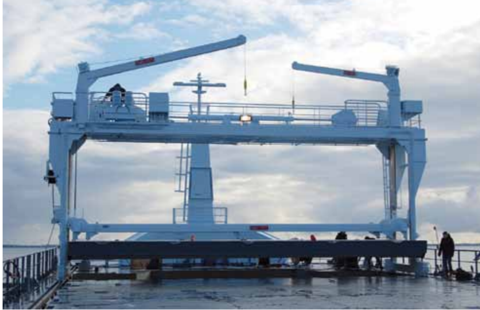
The upper deck shape allows for the 'Coops & Nieborg' hatch crane to be positioned at the forward end 'over the bow'
