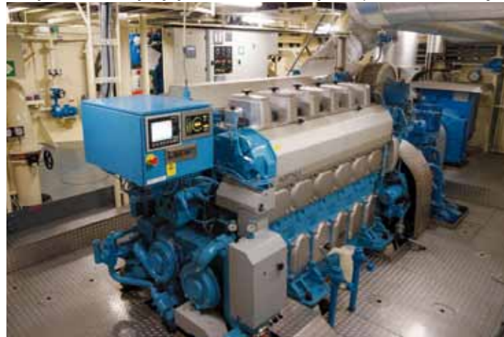
The ship has one controllable pitch propeller in a HD nozzle, which is powered by a Wärtsilä main diesel engine
