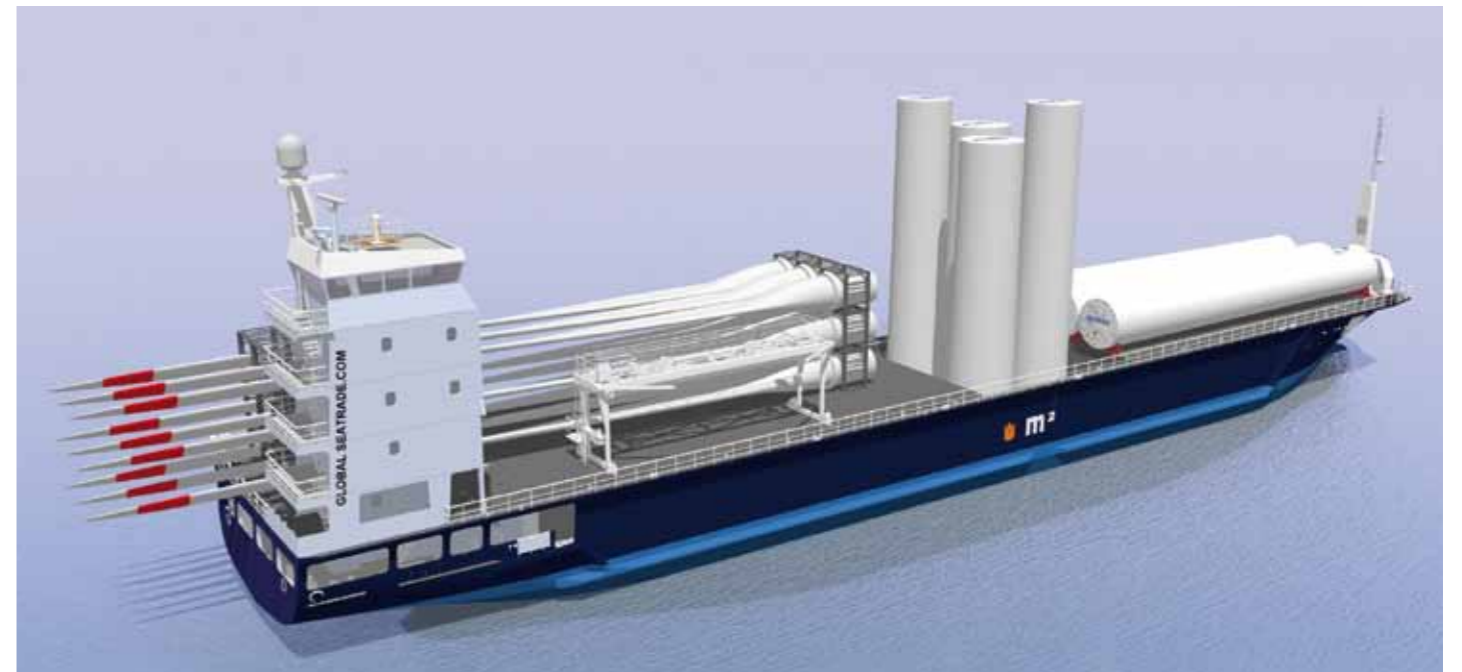
The shape and location of the accommodation provide a barrier-free cargo deck over the full length of the ship
