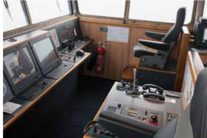
The wheelhouse contains the navigation console with all the required navigation and ship control facilities
