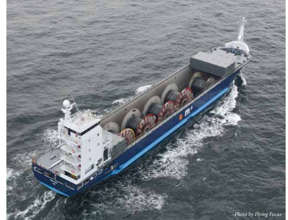
Nordic has an 'Open Top' notation and is suitable for cable laying, wherein the coils/reels are placed in the hold
